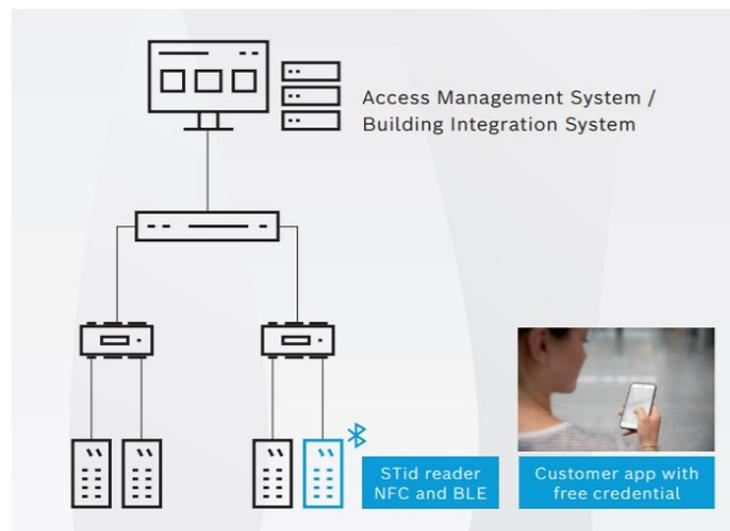
To use this solution, users must install the STid mobile app on their smartphone to receive a unique ID number. Then, when presenting their mobile phone to the reader, the authorization rights of the ID credential within the Access Management System or the Building Integration System will be checked by the AMC2 before access is granted.
